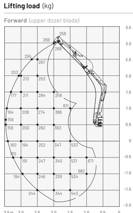
The loads in the diagram are within 87% of the hydraulic lifting load and within 75% of the tipping load.
