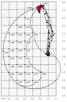
The loads in the diagrams (on the left) are within 87% of the hydraulic lifting load and within 75% of the tipping load.
