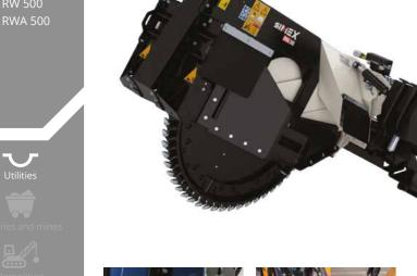
Designed for skid steer mounting, Simex RW and RWA wheel saws provide different solutions for working on hard or compact surfaces such as asphalt, concrete and rock: cutting and narrow trenches, set-section trenches, mini- and micro-trenches for fiber optic cable installation. Full protection of the wheel at any working depth guarantees maximum safety of persons and property.
