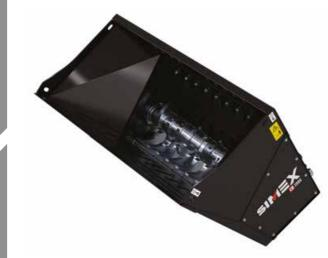
Designed to reduce the volume of aggregates and reinforced concrete directly on site, CB crusher buckets with rotor system give optimal performance when working with iron, rock, soil and deformable parts, and wet or humid materials. The exceptional cutting force allows any material to be crushed thanks to the rotor with teeth activated by high-displacement radial piston hydraulic motors in direct drive. Automatic system inverts rotation of the drum in case of blocking (Simex patent).
